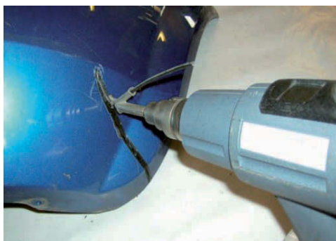
Fotod 11, 12, 13 – Plasti keevitamine erinevate meetoditega
